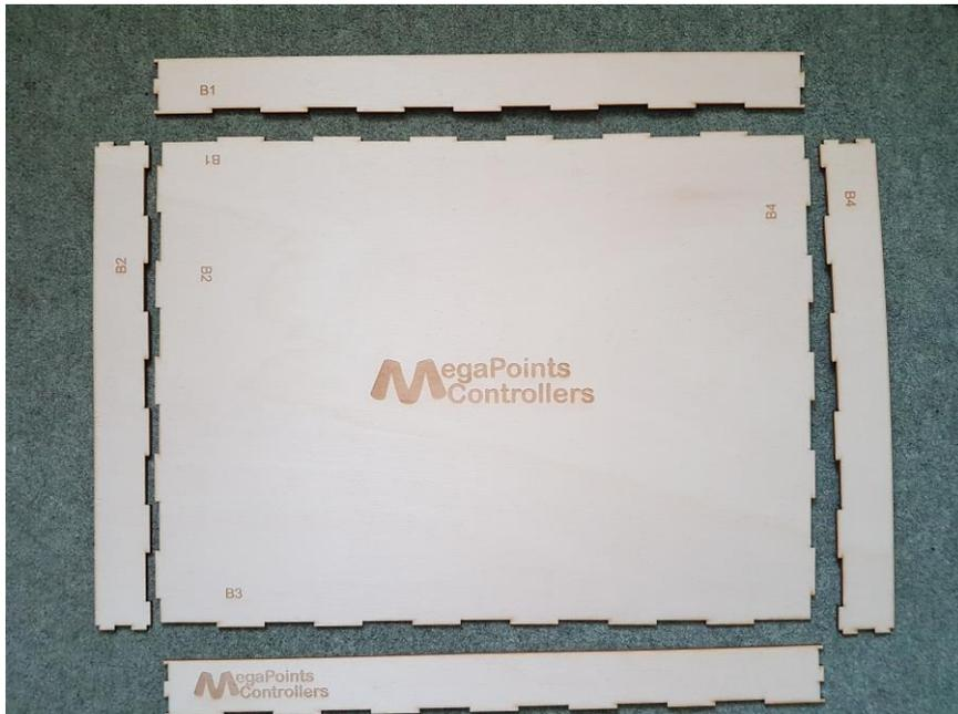
Turn the front panel over so the logo is facing down and apply wood glue to all facings. Don't forget the corners of the edge pieces.
