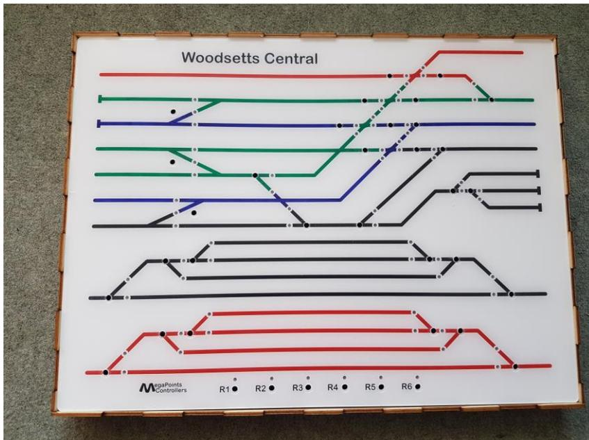
Check all edges to ensure it lies fully recessed and flat. Check the MDF backing is the right way around and matches the fascia ☺
